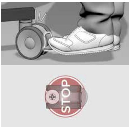
(fig.15b) Braking castors engaged.
