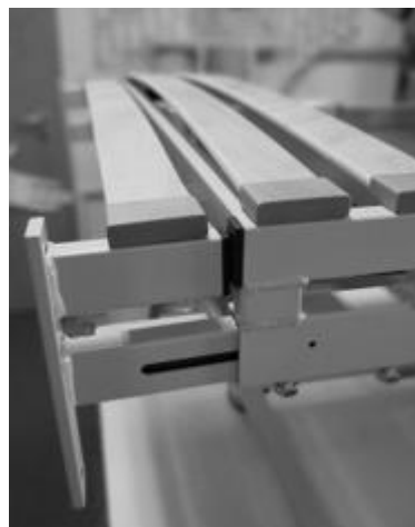
Figure 11: Assembly of the foot traverse (210 cm lying surface length)
